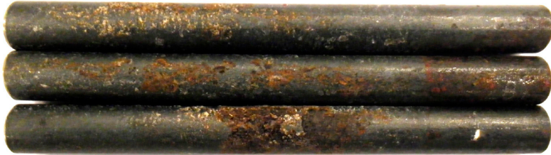
Figure 11. Corrosion products formed on the steel in mortar with 0.6% Cl exposed to dynamic moisture conditions.
