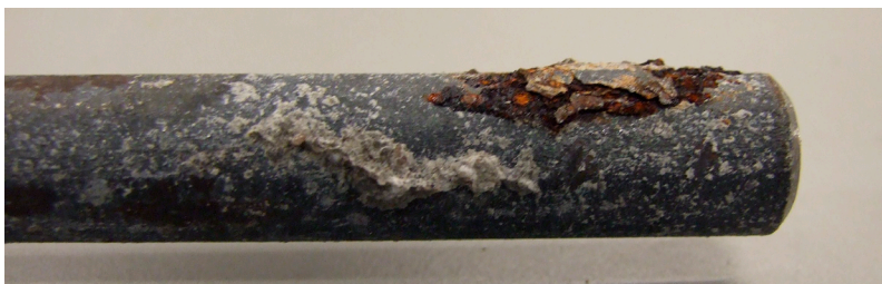
Figure 10: The surface of a steel sample cast in mortar with 1% Cl by mass of cement exposed to 97% RH. The figure shows that a part of the mill scale is detached from the steel surface probably due to formed corrosion products beneath the mill scale.
